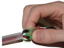
Then position the 4" piece of Shrink Tubing centered over the wrapped connections completely covering the stripped section. Use the Heat Gun or Blowtorch to shrink the tubing\*.
