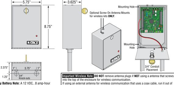
Standby Battery Note: A 12 VDC, .8 amp-hour battery (P/N 1801-008) can be used to supply standby power to a single tracker expansion board. If using an external antenna for wireless communication that uses a coax cable, run it out of the BOTTOM of the enclosure. DO NOT run coax cable out of the top of the enclosure, it will leak and cause damage to the circuit board.
