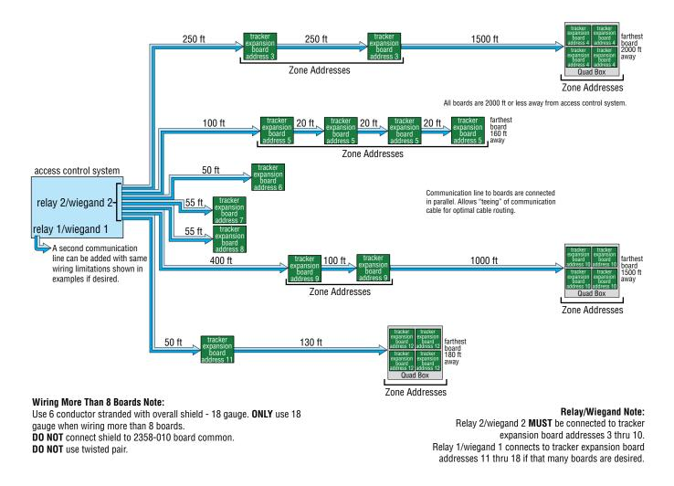
**IMPORTANT** Wireless communication maximum distances between the access control system and tracker expansion boards will vary from the HARDwire run distances illustrated above. See the instruction sheets in the wireless kits and the Layout and Start-Up Procedure for the correct distances between the hardware when using wireless communication.
