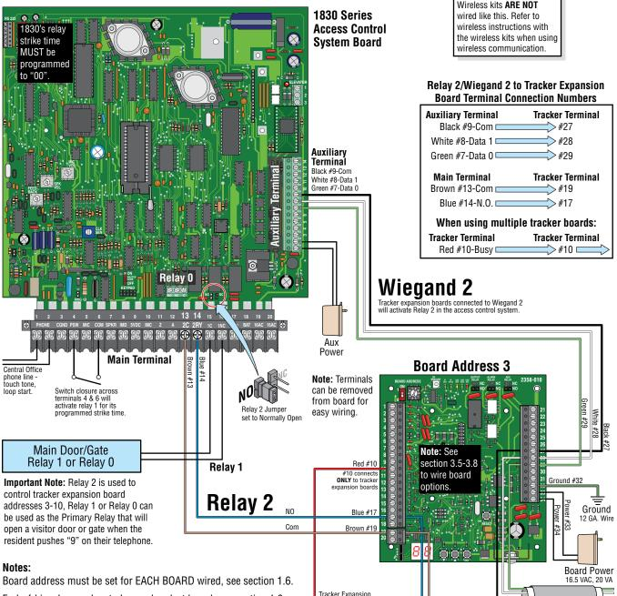
End-of-Line Jumper has to be used on last board, see section 1.8.
