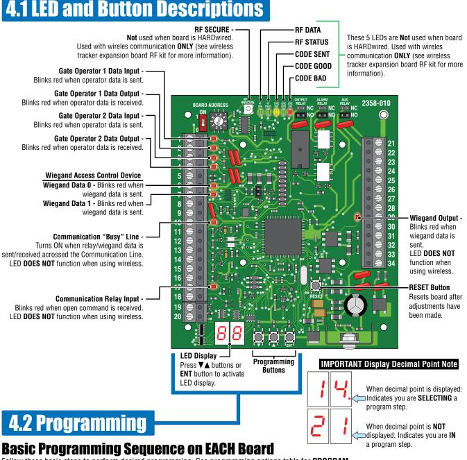
Follow these basic steps to perform desired programming, See programming options table for **PROGRAM STEPS** on next 2 pages. **EACH** tracker expansion board in the system **MUST** be physically programmed.
