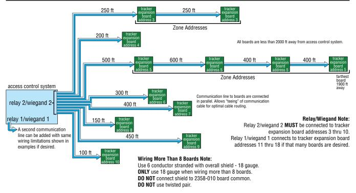
**IMPORTANT** Wireless communication maximum distances between the access control system and tracker expansion boards will vary from the HARDwire run distances illustrated above. See the instruction sheets in the wireless kits and the Layout and Start-Up Procedure for the correct distances between the hardware when using wireless communication.
