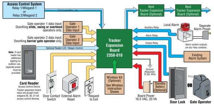
WARNING If the access control system is used to control a vehicular gate with an automatic gate operator, the access control device must be mounted a minimum of six (6) feet away from the gate and gate operator, ten (10) feet recommended, or in such a way that a person cannot operate the access control device and touch the gate or gate operator at the same time.
