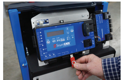
USB port for software updates and log files
